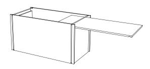
Slide the lid under the handles until the slots rest on the edges of the sides.
