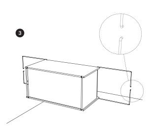
Attach the metal frame, make sure it sits in the slots and that the pins point outwards.
