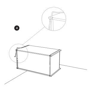
Push the frame slightly outwards while pulling it underneath the box and attach it in the two holes. Don't be afraid to bend out the frame when assembling so you do not damage the edges of the box.
