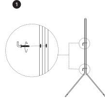
First make sure that the L-shaped screws are in place and prevent the two sides from coming apart.
