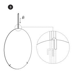
Lastly, place the mirror in the assembled frame. Make sure that the hook catches the L-shaped screw on the back so that the mirror cannot fall over.
