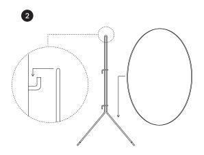
Afterwards fix the frame to the wall. Make sure that the hook is securely fixed to your wall. Please use a suitable dowel and choose a different hook if required.
